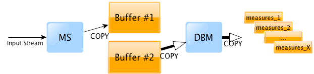
Figure 2 : The double-buffer method
